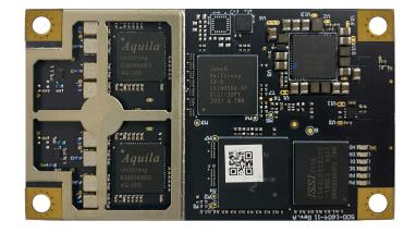
The Vega 34 is our most advanced GNSS heading and positioning board.
